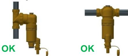
The swiveling part makes installation possible on pipes:
